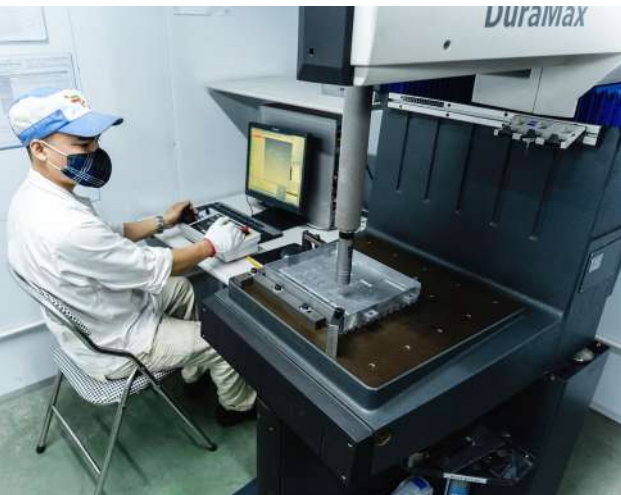
Measuring the dimensions of parts by CMM machine
